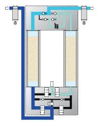
tion to adsorption is carried out after pressure has been built up. The change from regeneration to adsorption without an accompanying pressure surge is only possible if both vessels have the same working pressure. Duration of pressure build-up: 3 minutes.
